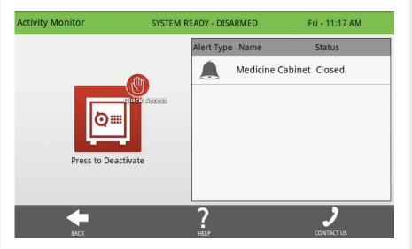
Activity monitoring sensors function independently from the intrusion security system on the IQ Panel. These sensors provide warning information via voice prompts and/or chimes. The warning notifications will be announced anytime that an activity monitoring sensor is opened or closed (or motion detected for motion sensors). These sensors are defined at the time of installation.
