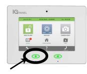
When you press the Emergency Button the Emergency Panic screen appears. Touching any of the buttons will trigger an alarm manually.
